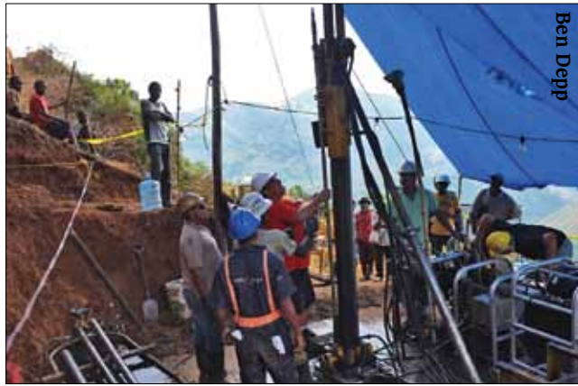
A Canadian with Haitian and Dominican workers at Newmont gold exploration site in Haiti’s north. Workers drilled 330 meters into a mountain to extract samples for testing. Three Dominicans and a half dozen Haitian workers help remove the pipes through which samples were collected
